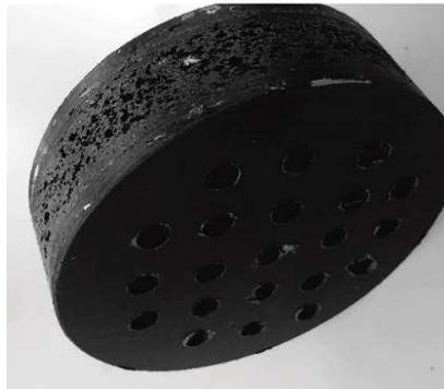
Fig. 2. Array of the HR formed on the surface after drilling holes [5]
